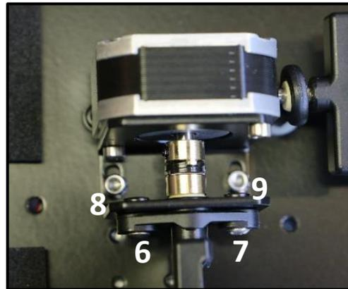
FIGURE 78: REMOVE THE TILT MIRROR FIXATION
