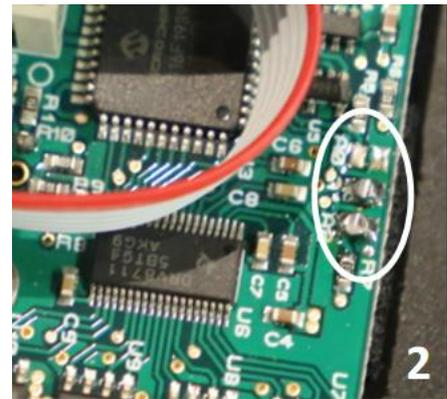
**FIGURE 83: STEPPER MOTOR BOARD ADDRESSING PIN**
