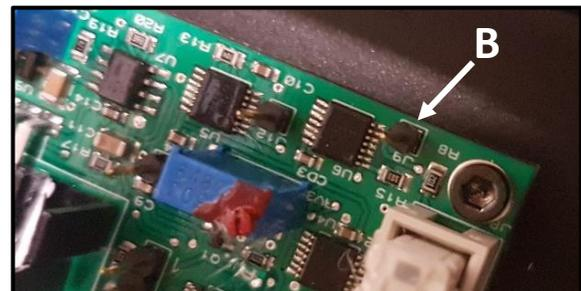
FIGURE 60: SCANNING MIRROR SENSOR SIGNAL PINOUT (FROM THE BOARD)
