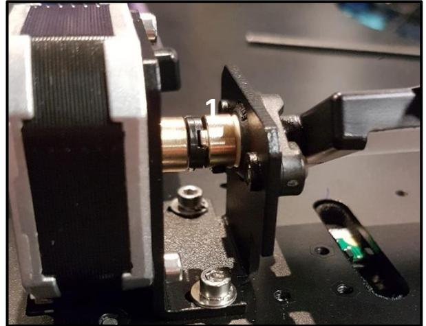
FIGURE 74: ADJUSTMENT OF THE MOTOR-MIRROR COUPLING
