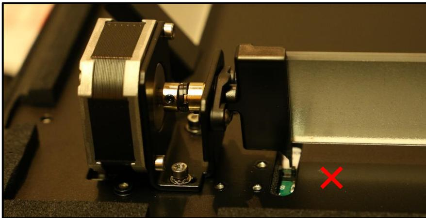
FIGURE 75: BAD TILT DETECTOR PIN POSITION
