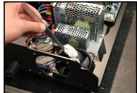
FIGURE 93: FAN BLADES CLEANING
