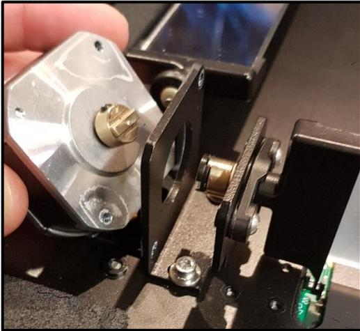
FIGURE 73: NEW STEPPER MOTOR ASSEMBLY
