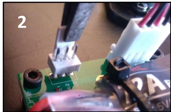
FIGURE 57: REMOVE THE POLARIZER
