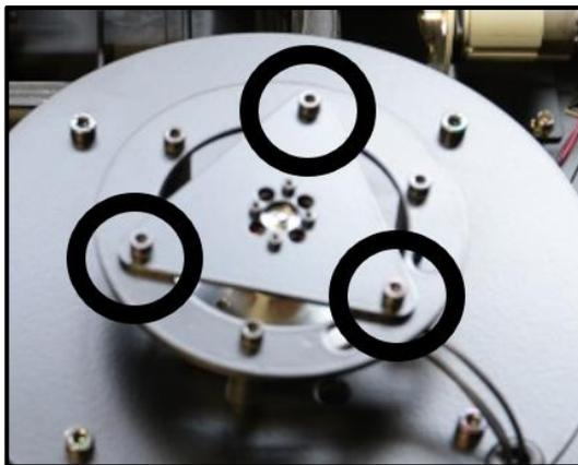
FIGURE 88: SCANNING MIRROR REMOVING
