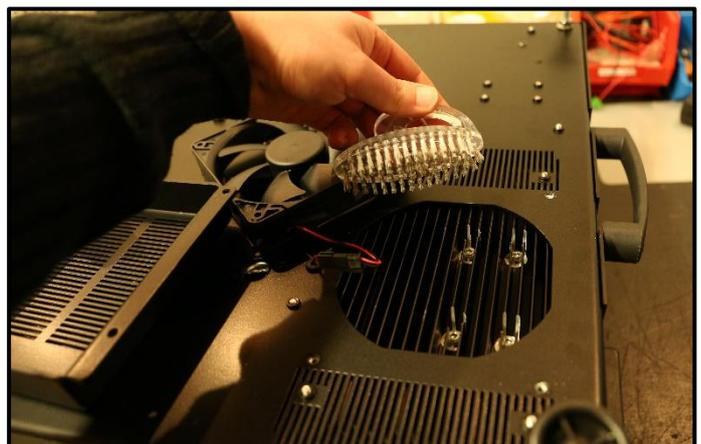
FIGURE 95: HEATSINK CLEANING
