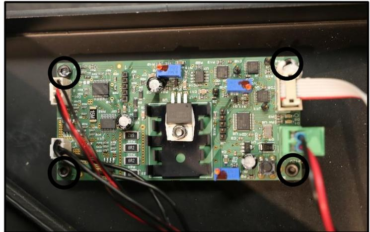
FIGURE 49: SCANNING MIRROR BOARD REMOVING
