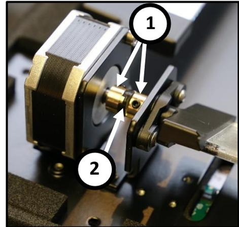
FIGURE 68: MOTOR-MIRROR COUPLING PARTS
