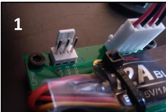
FIGURE 56: REMOVE SCANNING MIRROR CABLE
