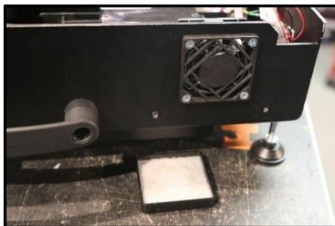
FIGURE 92: UNSCREW THE FILTER HANDLER
