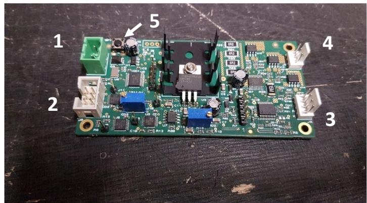
FIGURE 50: SCANNING MOTOR BOARD WIRING
