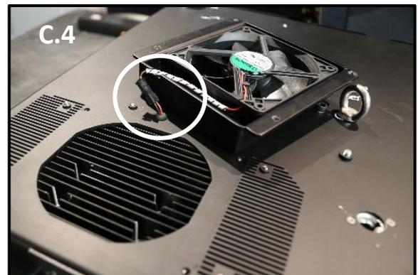
FIGURE 44: FAN CONNECTOR
