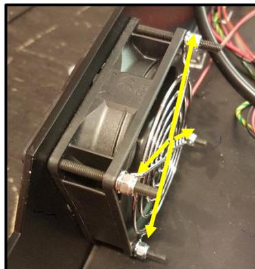
FIGURE 40: EXHAUST FAN REMOVING
