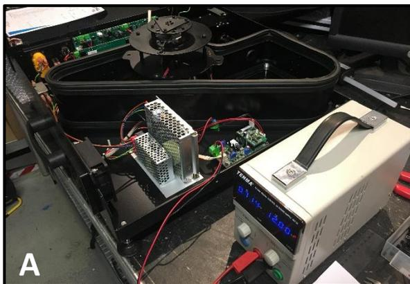
FIGURE 52: EXTERNAL +12VDC POWERING
