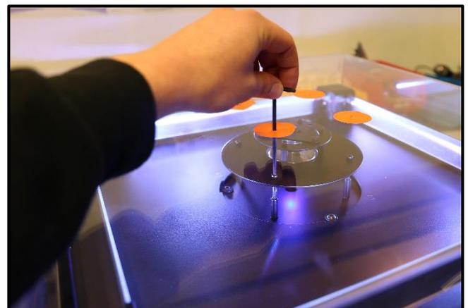
FIGURE 23 : PLATE LEVEL ADJUSTMENT
