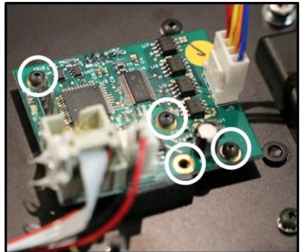
FIGURE 82: STEPPER MOTOR BOARD REPLACEMENT
