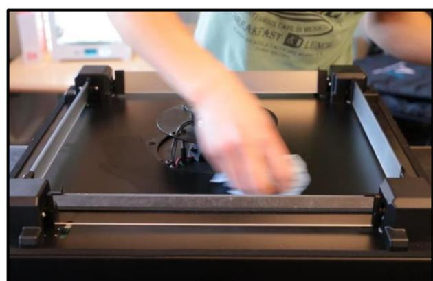
FIGURE 97: TILT MIRROR CLEANING
