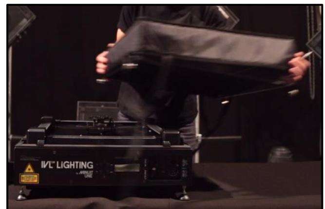
FIGURE 17 : REMOVING SQUARE PLEXIGLAS SHAPE (4/4)
