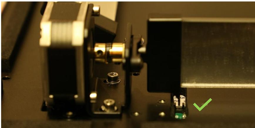
FIGURE 76: GOOD TILT DETECTOR PIN POSITION
