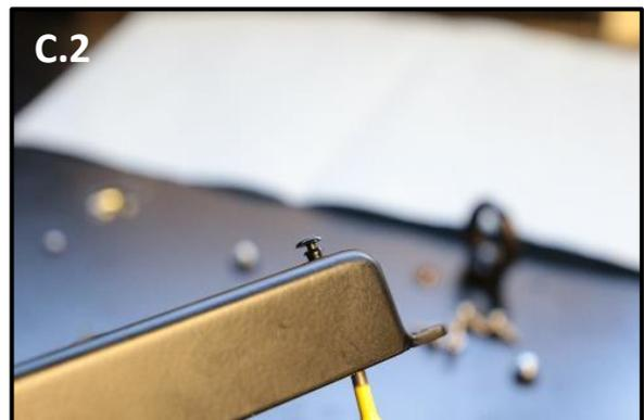
FIGURE 42: REMOVE THE PIN
