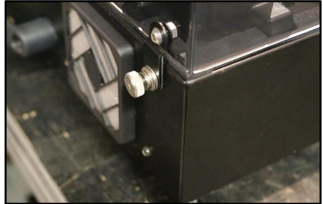
FIGURE 15 : REMOVING SQUARE PLEXIGLAS SHAPE (2/4)
